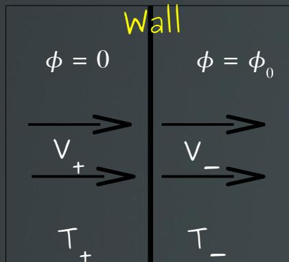
$$\begin{aligned} w_+ v_+^2 \gamma_+^2 + p_+ - V_0(0) &= w_- v_-^2 \gamma_-^2 + p_- - V_0(\phi_0) \\ w_+ v_+ \gamma_+^2 &= w_- v_- \gamma_-^2 \end{aligned}$$
